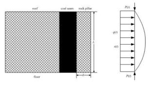
Fig. 1. Simplified model of coal and rock mass
